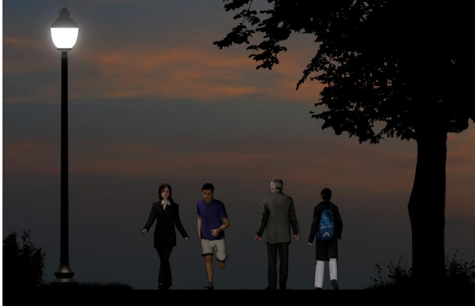
Rendering 2 – Depiction of Minimum Vertical Illuminance (50 foot light pole spacing)
