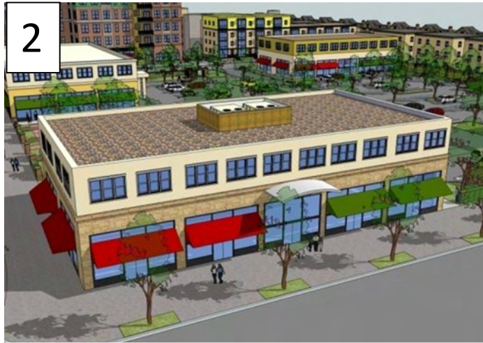
Where possible locate HVAC units on the building roof and appropriately screen them.
