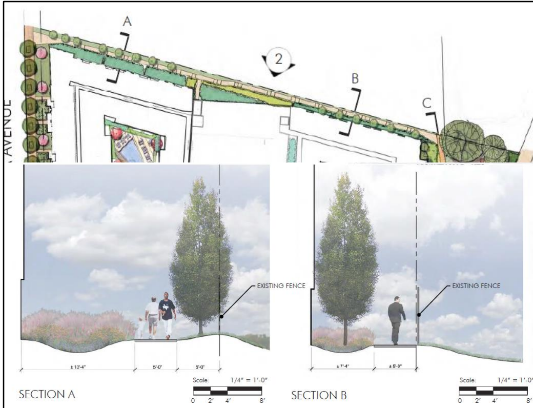
Section details of the proposed east-west pedestrian connection along the northern property line
