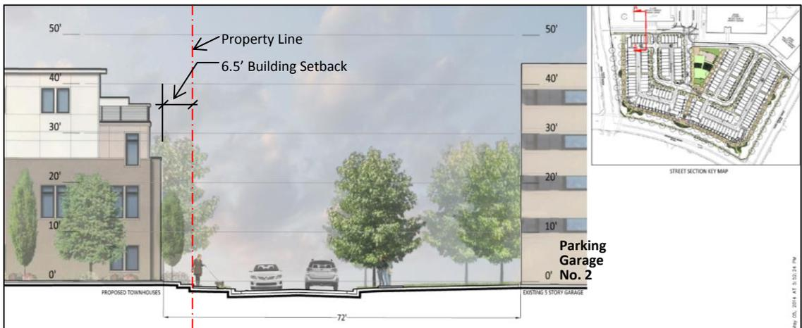
*Cross section illustrating the conditions of the waiver request*
