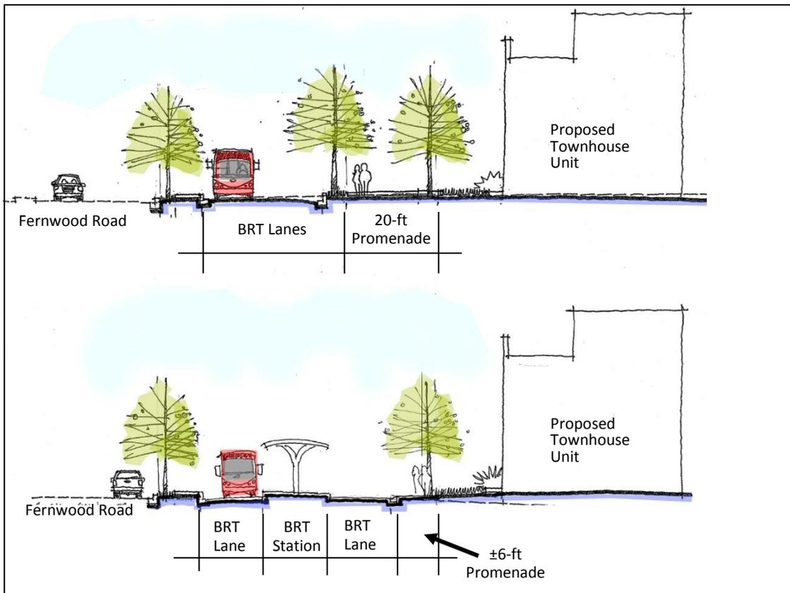
Cross Sections illustrating potential conditions with an implemented BRT System. The illustration (top) shows bus travel lanes adjacent to the proposed 20-foot promenade. The illustration (bottom) shows bus travel lanes and a potential station with a reduced promenade.
