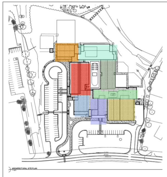
Plan analysis illustrates the shifted 9-Square, program element relationships and the pivotal form of the central open “square.”
