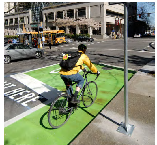
Intersection improvement with bike boxes Portland, OR
