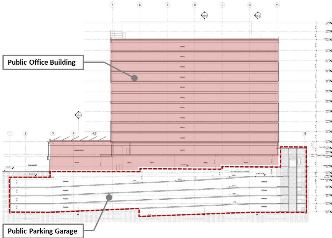
Figure 4: Proposed Public Office Building Section
