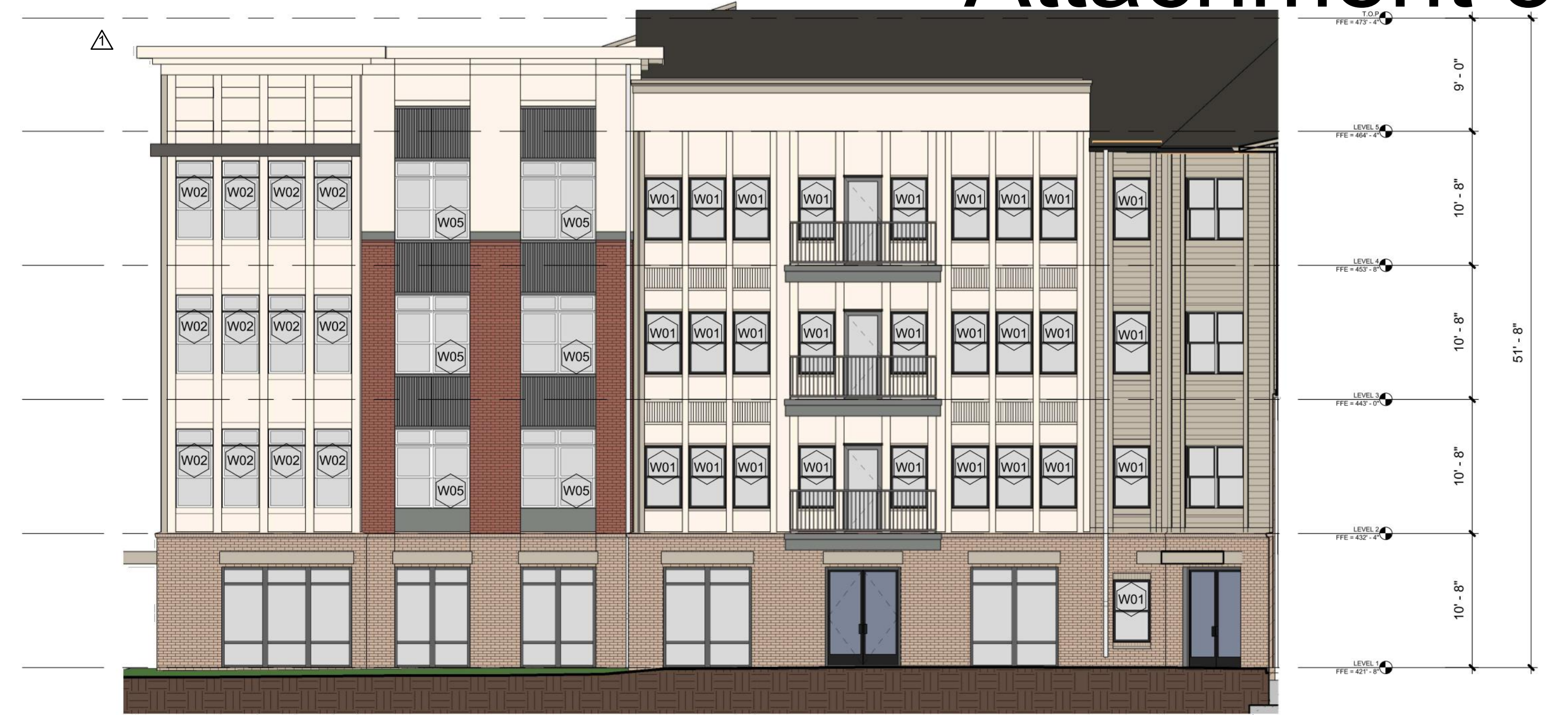
2 BLDG 3000 SOUTH ELEVATION 1/8" = 1'-0"
