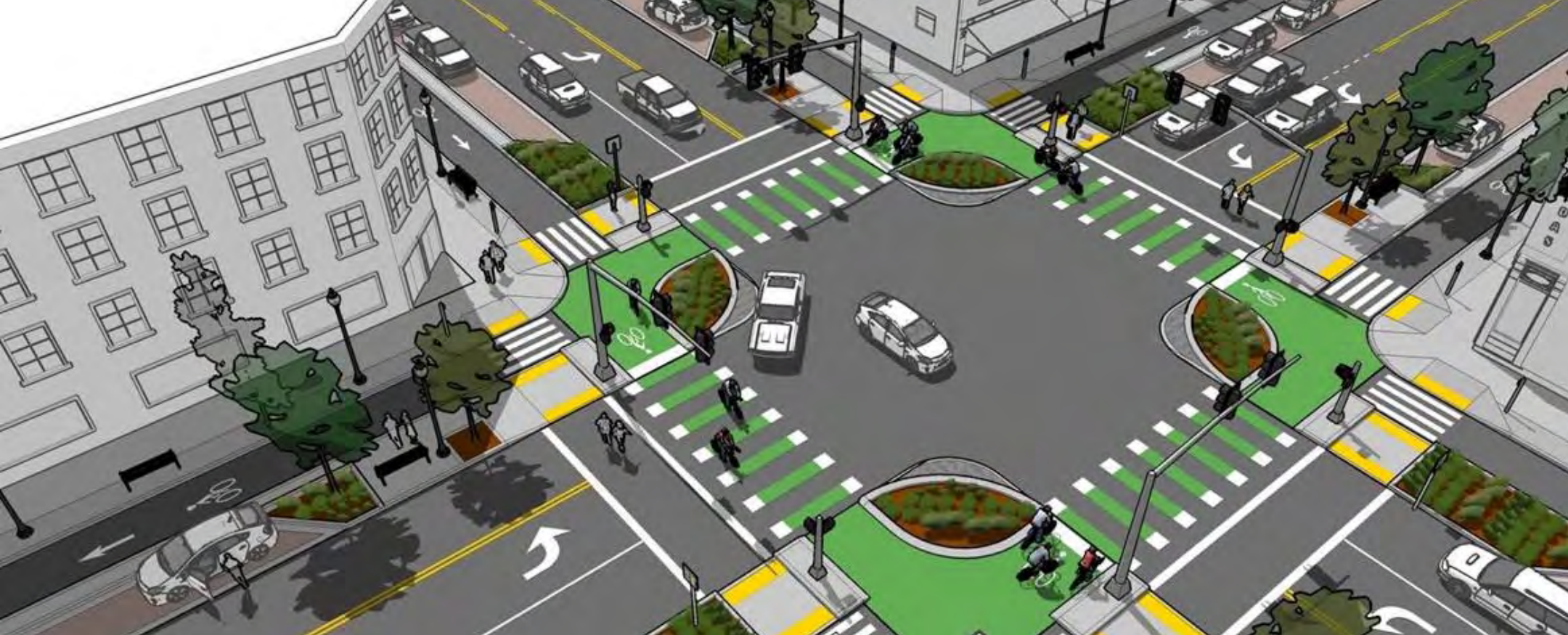
Figure 17: Protected Intersection Illustrative
