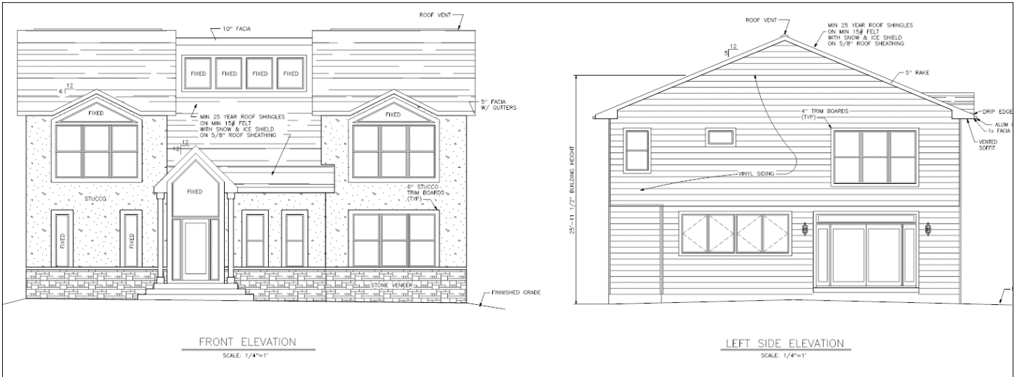
Figure 8: Detached house elevation
