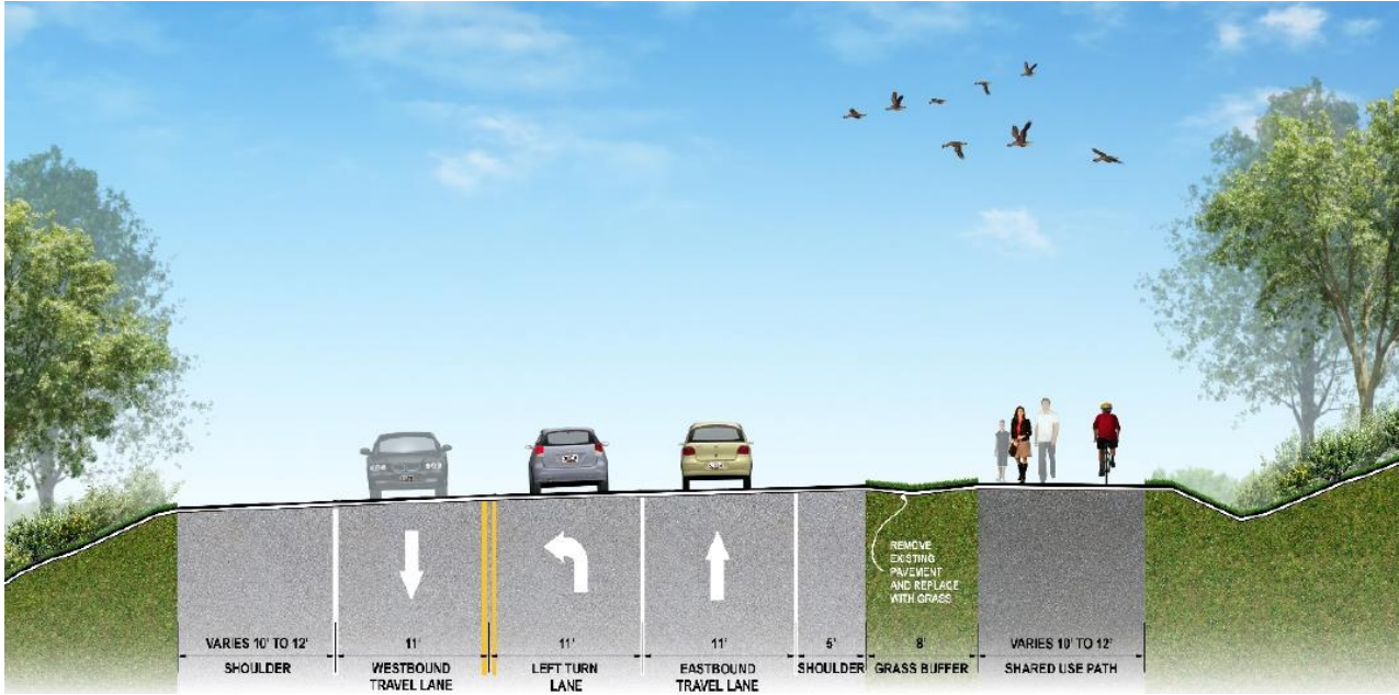
Figure 9: Muncaster Mill Road Cross Section
