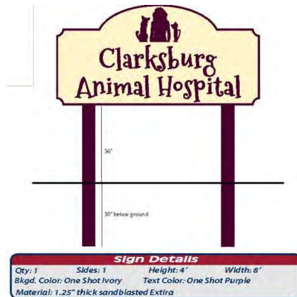
SIGN A. SIGN TO BE MOUNTED ON 4"X4" POSTS.
