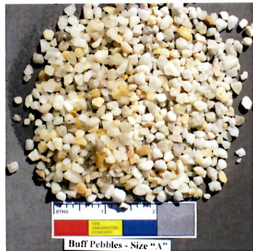
Earley Process pebbles screened to one size
