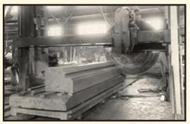
Large stone-cutting machine at Fuller Plant
