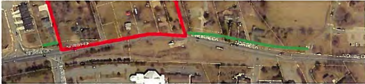
Figure 1 - Critical gaps in the existing sidewalk system on the north side of Norbeck Road highlighted in green.
