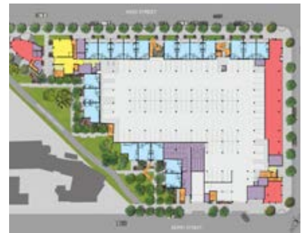
This floor plan shows structured parking screened by housing and retail uses facing the streets.
