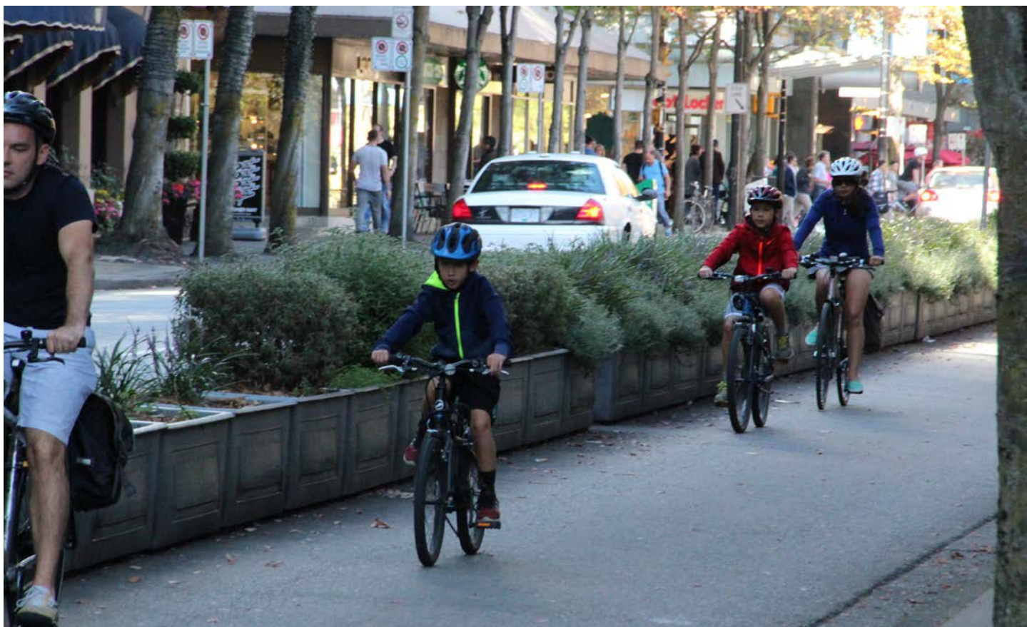
Planters provide separation from traffic for these separated bike lanes in Vancouver, British Columbia.
