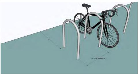
Minimum Dimensions for short-term bicycle parking perpendicular to the curb.
