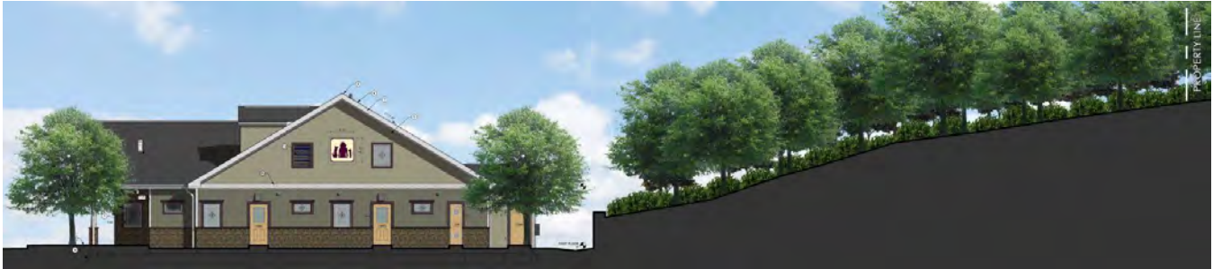
Figure 6. South elevation showing retaining wall and reforested/forested area to the east of the building extending to the property line. A similar retaining wall is proposed to the north of the building.
