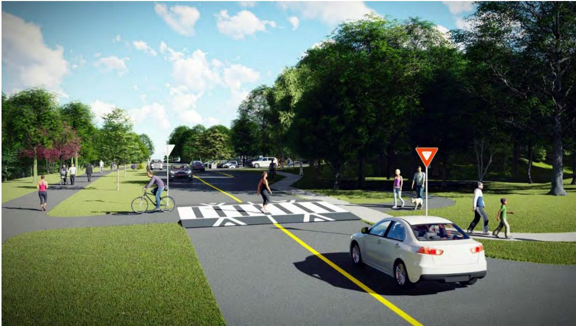
Figure 6: Alternative A - Permanent Road Diet with speed table looking north approaching the CCT (rendering by Floura Teeter)
