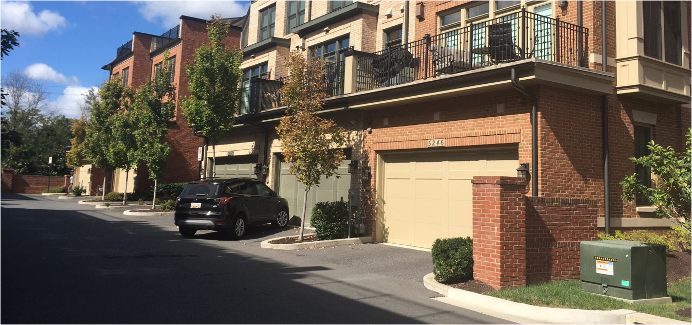
Figure 3.18: Alleyways shall be a minimum of 40 feet wide when townhouse window sills are greater than 27ft in height
