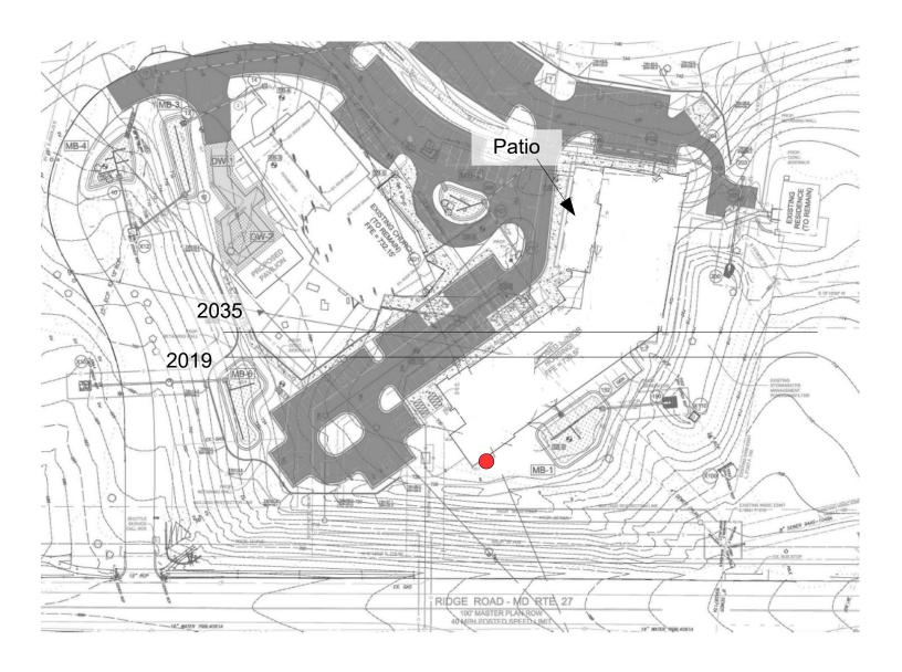
Figure 1: Site Plan with Primary Noise Assessment Location ( ) and Unmitigated 65 DNL Noise Contours 2019 and 2035
