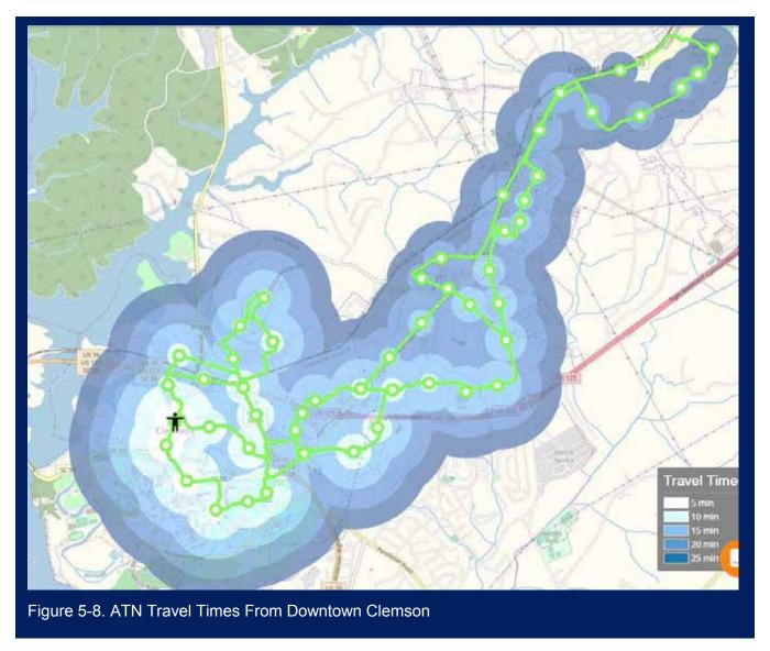
Figure 5-8 shows the travel times from Downtown Clemson on the ATN system. All stations can be reached in less than 21 minutes. The entire area within the dark blue outline can be reached in 25 minutes with a combination of riding and walking.
