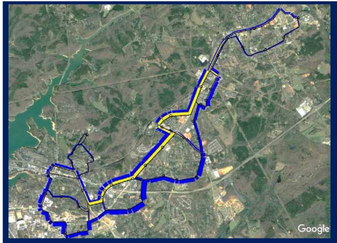
Figure 5-6. Guideway Loading. Blue represents occupied vehicles, yellow represents empty vehicles.
