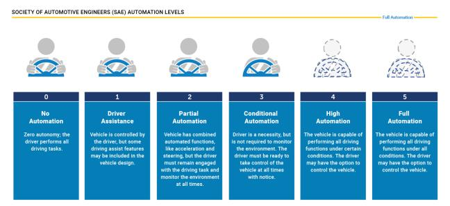
Technological advancements in the driverless car/personal automobile spectrum are also anticipated to benefit the Autonomous Transit spectrum as well. As Level 4 technology is refined, it is expected to be applicable to a wide variety of transit applications, including a range of vehicle sizes. Therefore, it is not expected that vehicle size or configuration will be a limiting factor when the technology reaches maturity.
