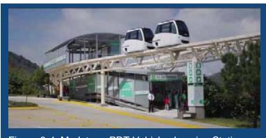
Figure 3-4. Modutram PRT Vehicles Leaving Station
