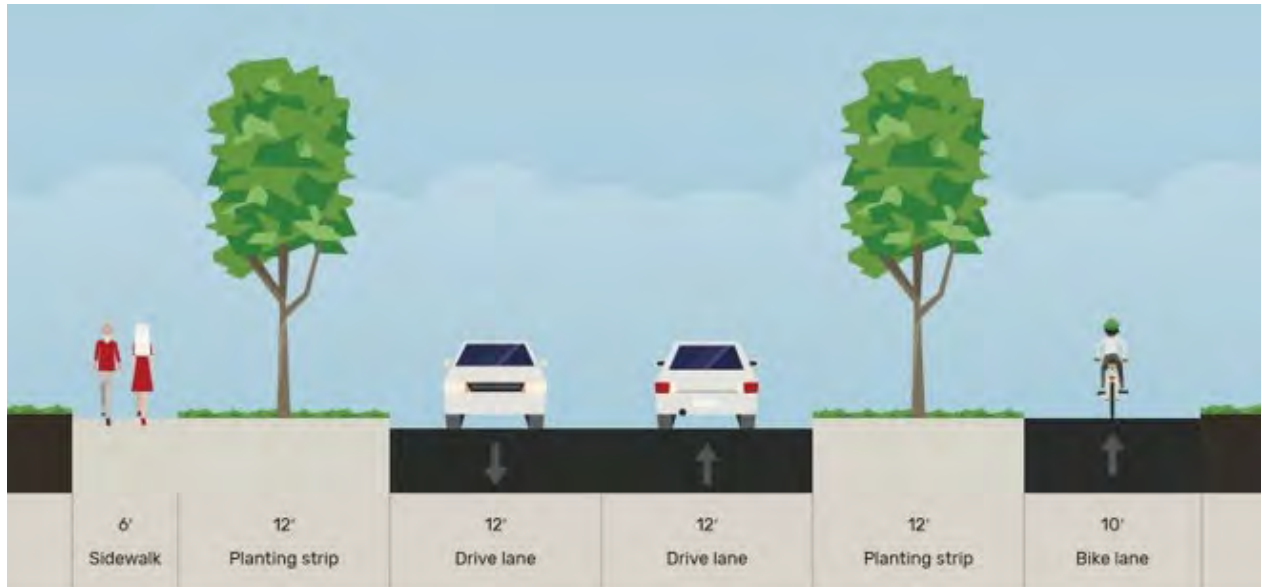
Figure 8: Crabbs Branch Way Extension – Cross Section
