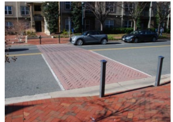
Figure 48: Midblock crosswalks should be raised or constructed with specialized pavers to alert motorists that pedestrians may be crossing.
