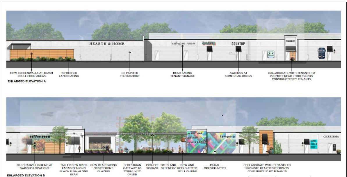
Figure 7 – Architectural Elevation of the rear of the existing shopping center with the new centralized open space
