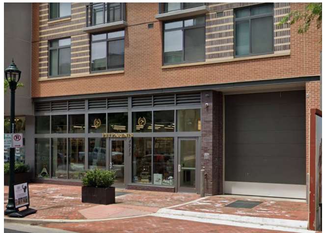
At these service entrances in Bethesda, the sidewalk materials are carried across the driveway entrance so the pedestrian experience is continuous.
