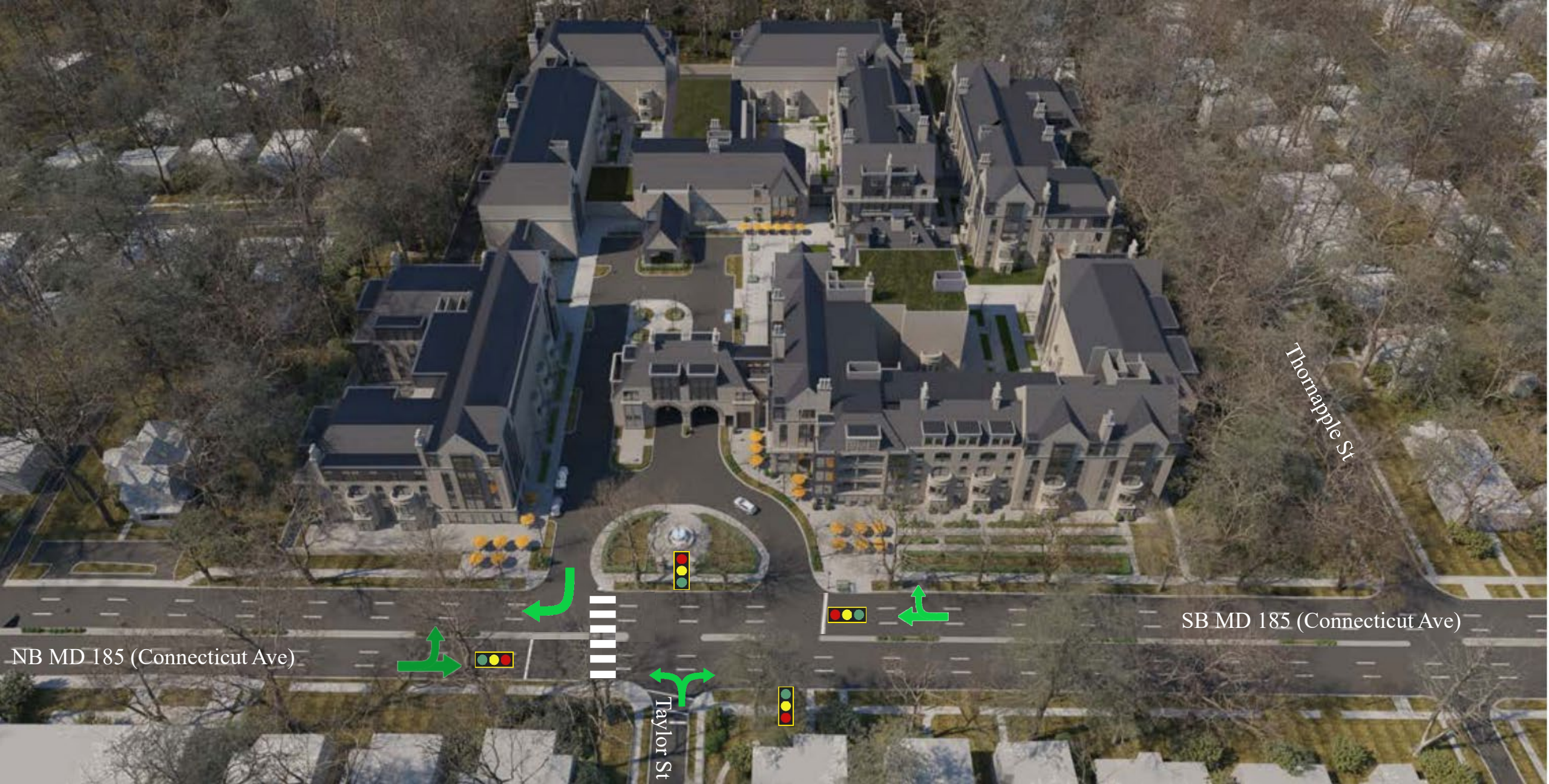
MD 185 (Connecticut Ave) at Taylor St – Signal Design Concept – Split Phase Alternative 2
