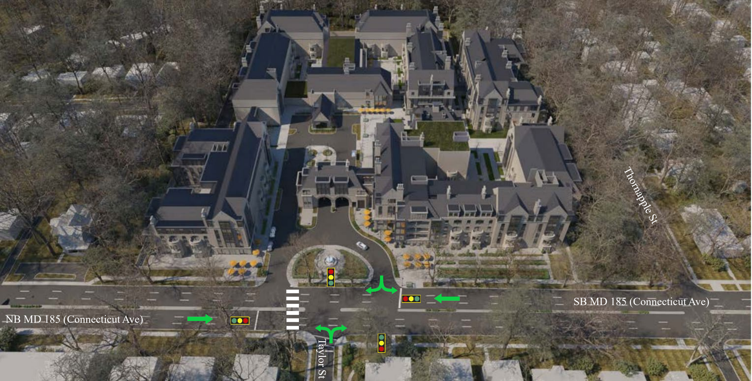
MD 185 (Connecticut Ave) at Taylor St – Signal Design Concept – Split Phase Alternative 1
