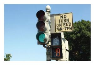
A sign next to a traffic signal indicates that no vehicles may turn right on a red signal between 7 a.m. and 7 p.m.
