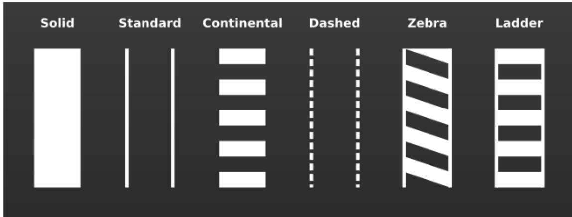
The ladder crosswalk markings on the far right can be compared with the continental and standard markings. Image Credit: SF Better Streets
