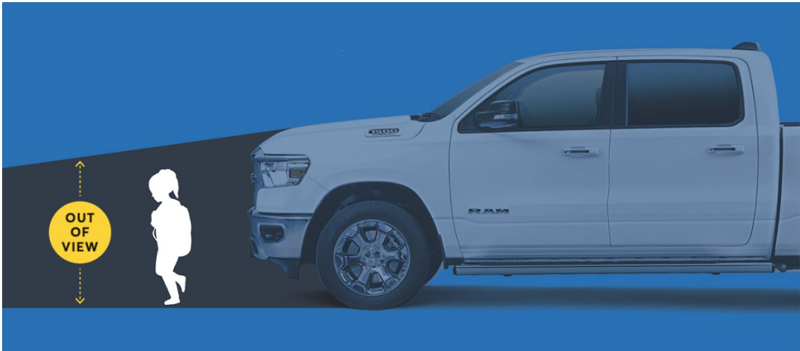
A truck and its front blind spot. Image Credit: Consumer Reports
