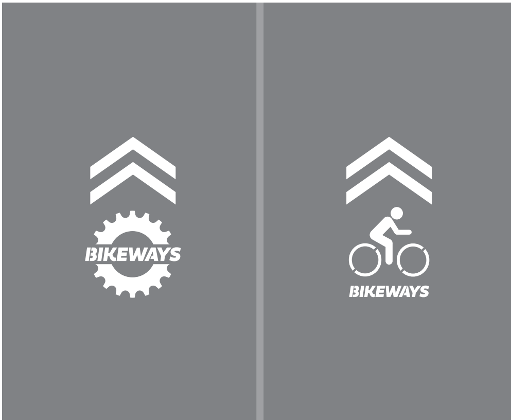
ROUTE MARKER PAVEMENT MARKING
