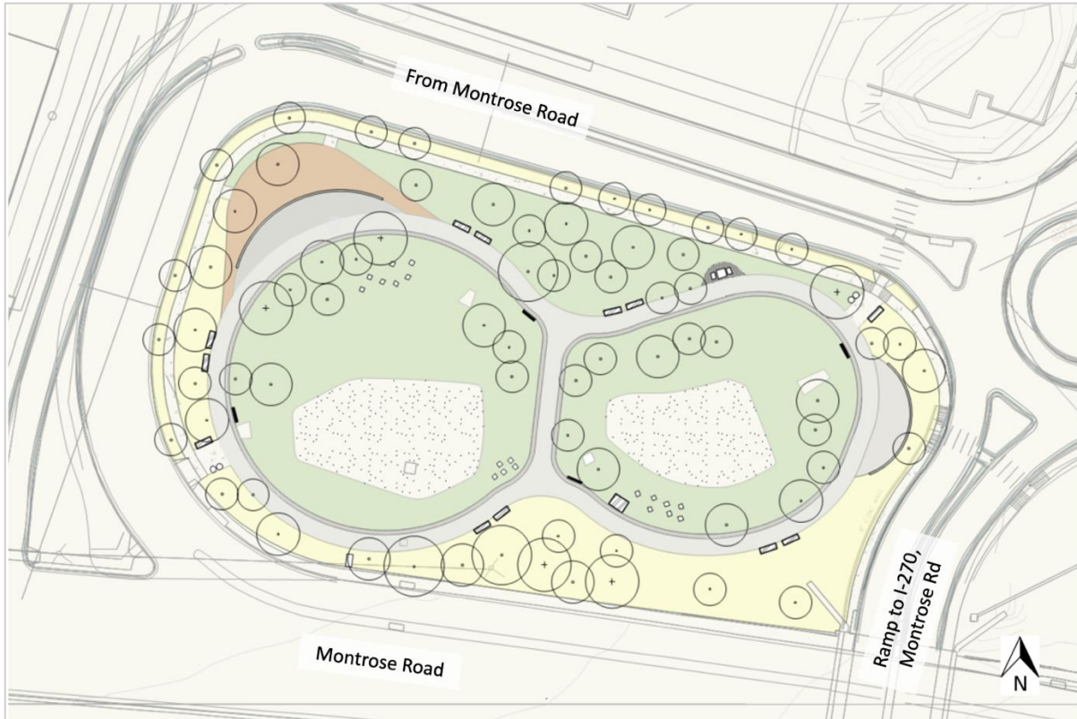
Figure 15 – Rendering of expanded public open space and new recreation amenities at an existing stormwater management facility with walking path, playscape, fitness elements, seating, bioretention plantings, and trees
