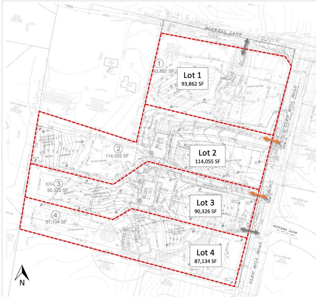
Figure 4 - Proposed Preliminary Plan with four lots; new driveways (orange arrows) and existing driveways (gray arrows).
