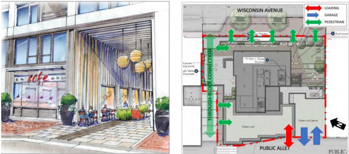
Figure 10 – Rendering (left) and Planview (right) of approved through-block connection for 7000 Wisconsin Avenue
