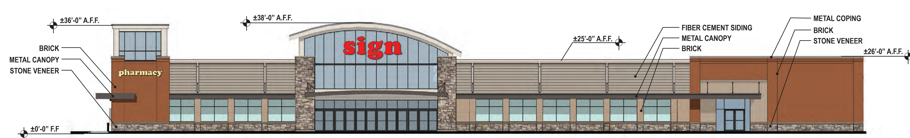
BUILDING 4 EAST ELEVATION
