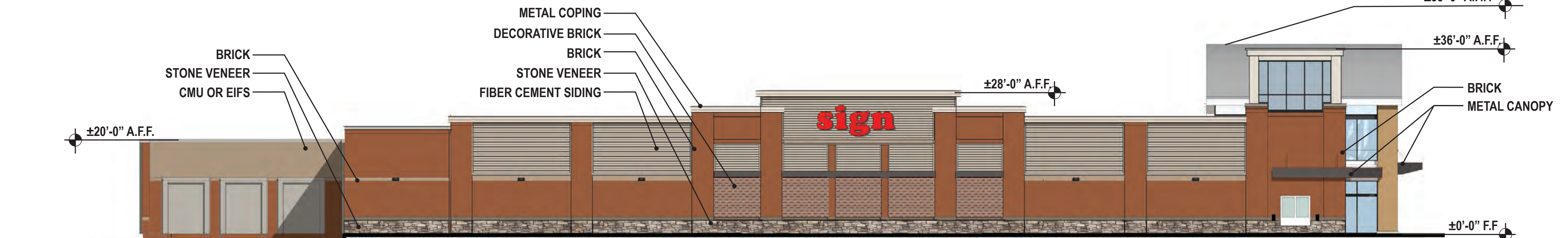
BUILDING 4 SOUTH ELEVATION
