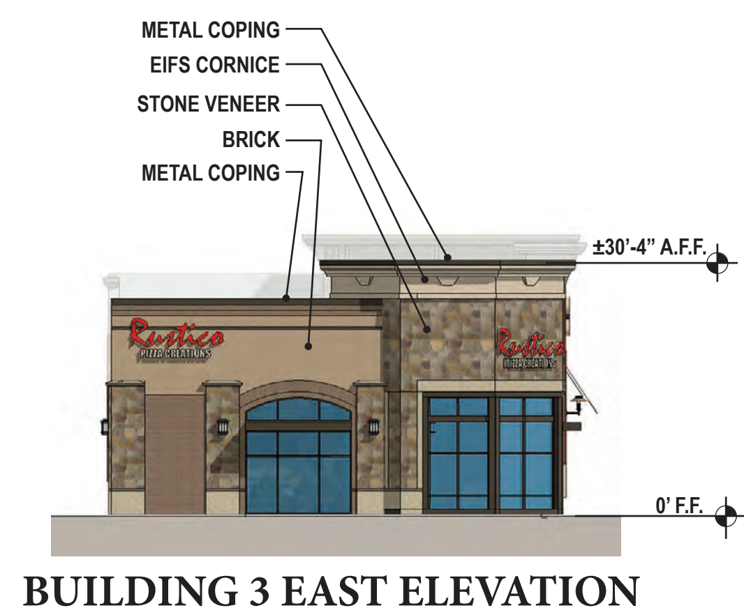
BUILDING 3 EAST ELEVATION
