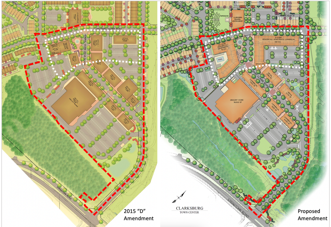
Figure 6 - Renderings of the approved 2015 Site Plan Amendment (82007022D) (left) and proposed site plan amendment (right). The dotted white boundary identifies the location of prior office space (left) and the proposed residential units (right). Other buildings, uses and layout in the proposed amendment are substantially similar to the 2015 amendment.
