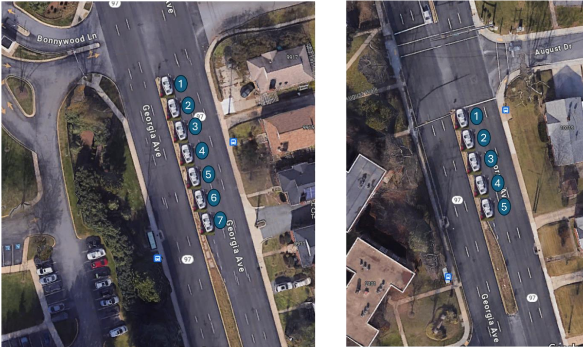
Figure 2: Left - left turn/u-turn storage at Tilton and Georgia. Right - u-turn storage at August Drive and Georgia Ave
