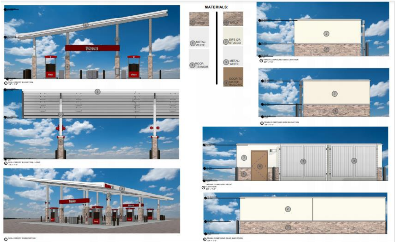
Figure 7: Fuel Pump Canopy and Trash Enclosure
