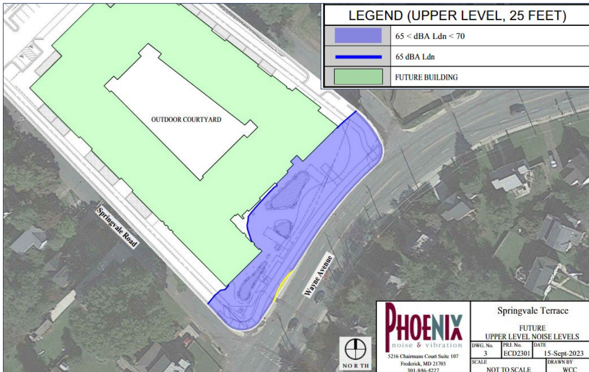
Figure 12: Wayne Avenue Noise Impacts
