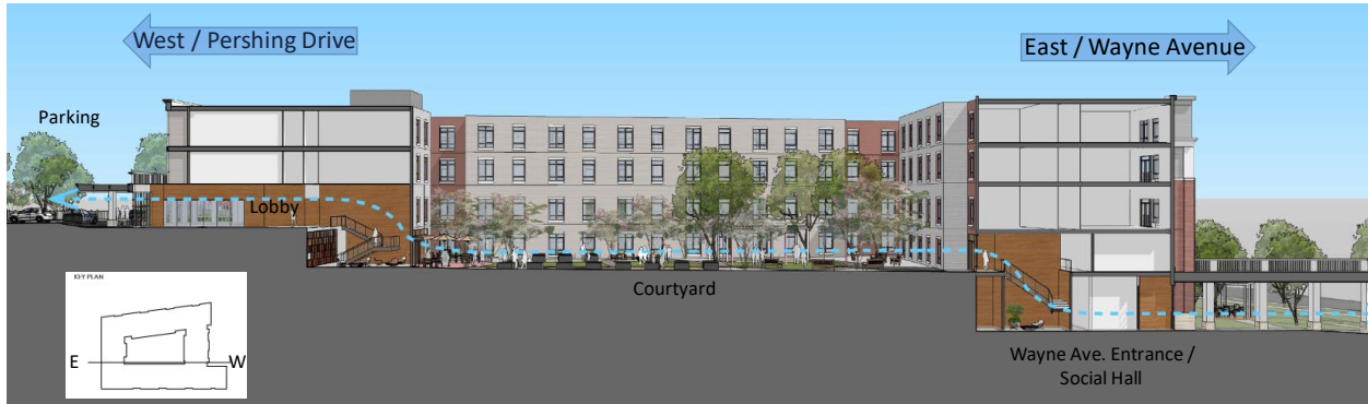
Figure 8 – East/West Building Section
