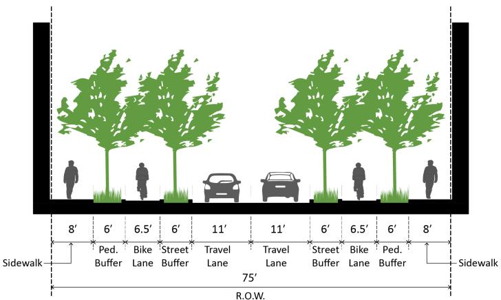
**Town Center Street** | 2 travel lane section Proposed Section: One-way separated bike lane both sides
