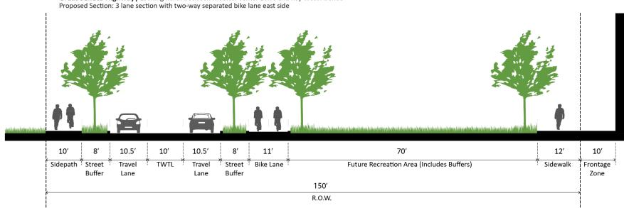
**Great Seneca Highway** Looking north between Medical Center Drive and Key West Avenue Proposed Section: 3 lane section with two-way separated bike lane east side
