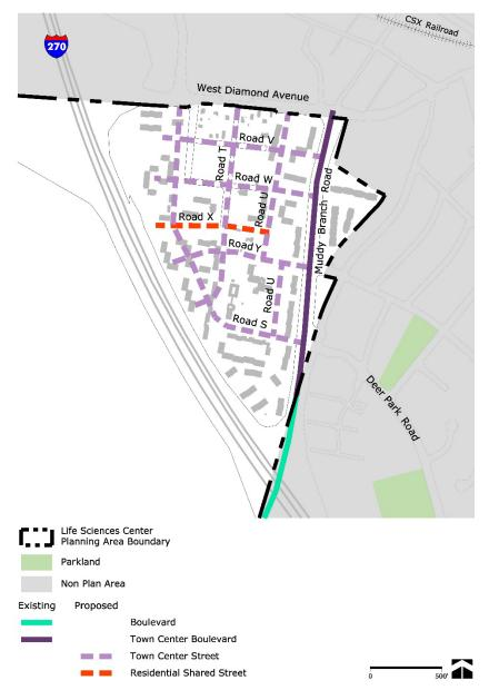
\* As illustrated, Road U is offset across Road Y to reflect the existing development pattern. If redevelopment of multiple properties is possible, a configuration that aligns Road U across Road Y would be preferred.
