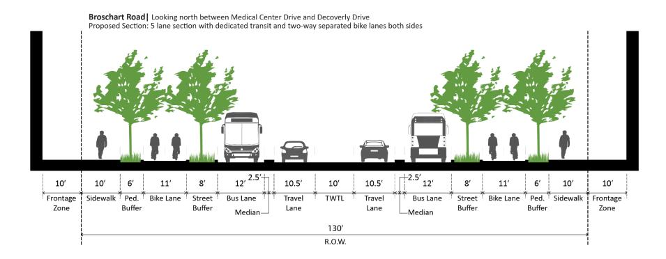
Figure 25: Broschart Road Cross-Section
