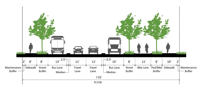
Figure 29: Muddy Branch Road Cross-Section
