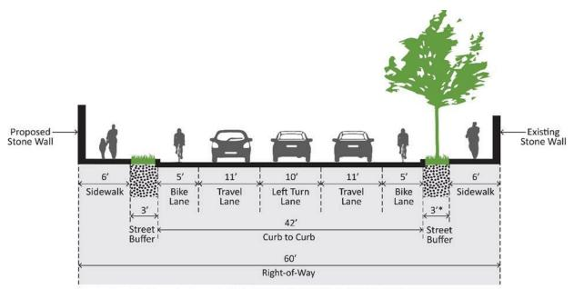
\*Note: Street Buffer varies from 0' – 30,' with the wider sections allowing for a larger street buffer and bike lane based on the complete streets design standard.
