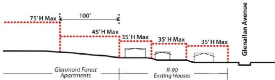
Figure 7: Eastern Transition Zone
