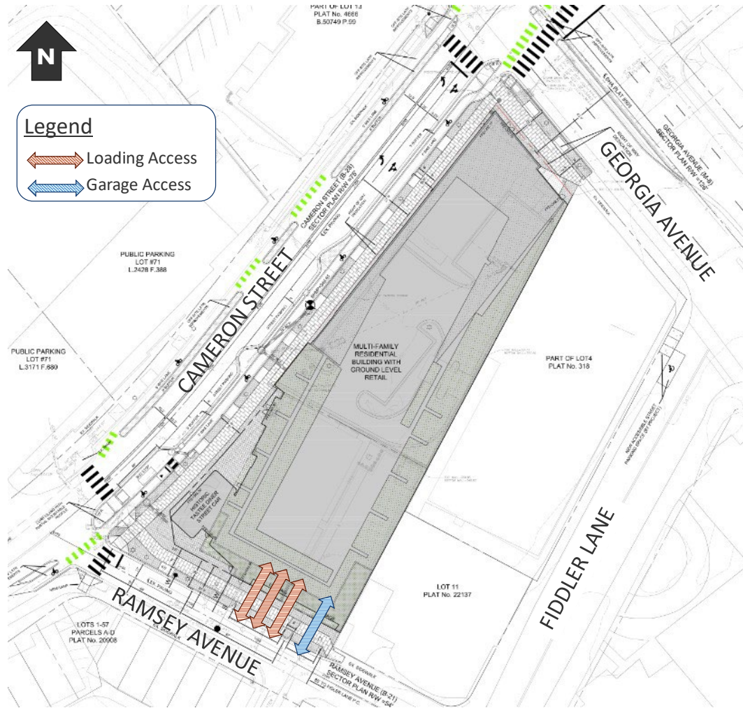
Figure 12: Site Access and Circulation
