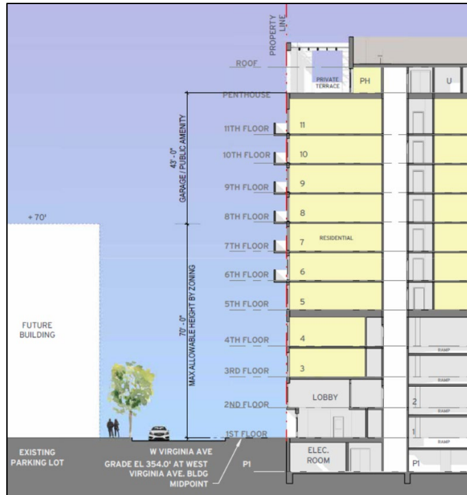
Figure 9 – Diagram showing above grade parking due to Major Public Facility (public park)
