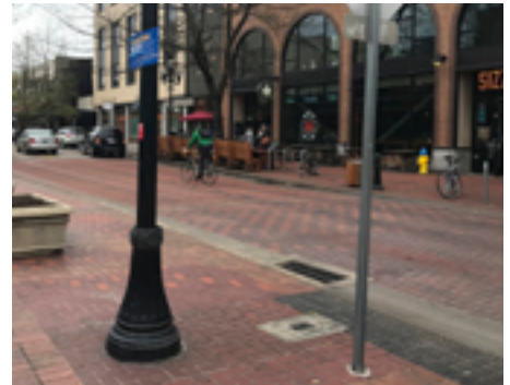
Figure 21. Example of Curbless Streets in Denver, CO,; West Palm Beach, FL; and Eugene, OR, where the travel lane and zones are defined by planters, bollards, and other furniture elements.
