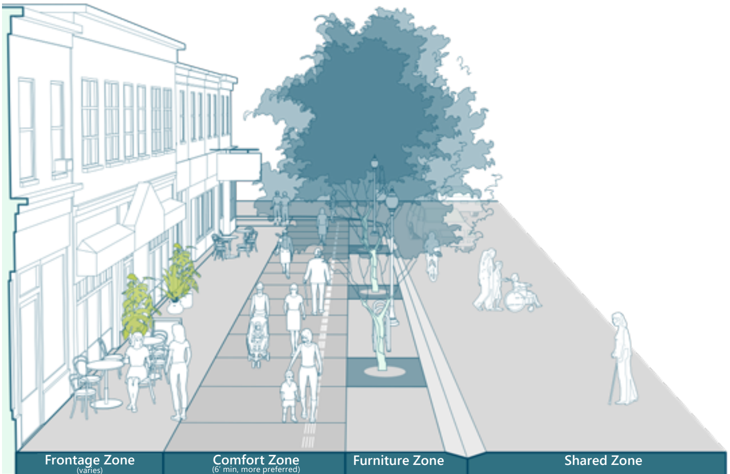
Figure 11. Zones of a Curbless and Shared Street
