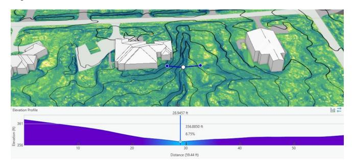
Figure 3. 3D Model: Stream Morphology Analysis, Cross section
