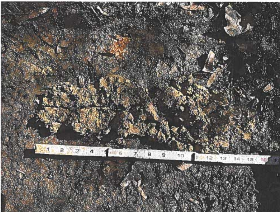
6. View of non-hydric soil profile obtained from dry ephemeral channel (03/20/2024).
