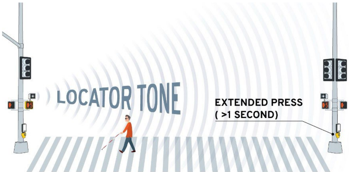
Figure 52: Illustration of how audible beacons work (Source: Polara)
