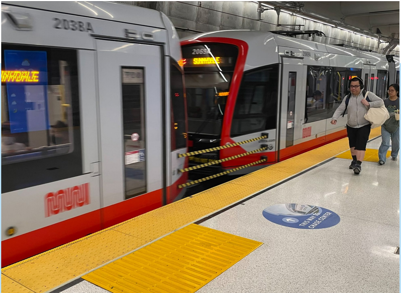
Figure 15: Example of transit door location TDIs
