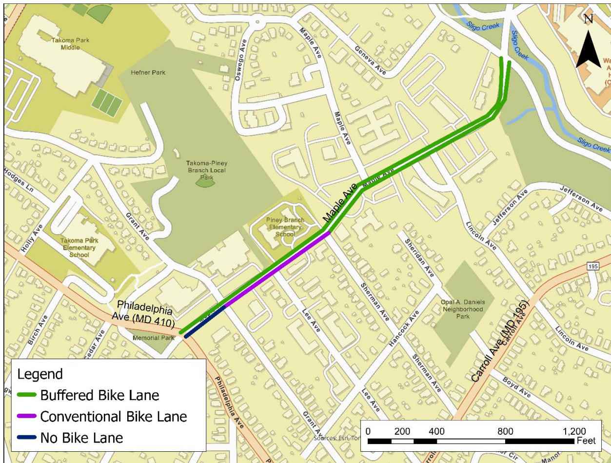
Figure 16: Schematic of Proposed Bike Lane Facility Types
