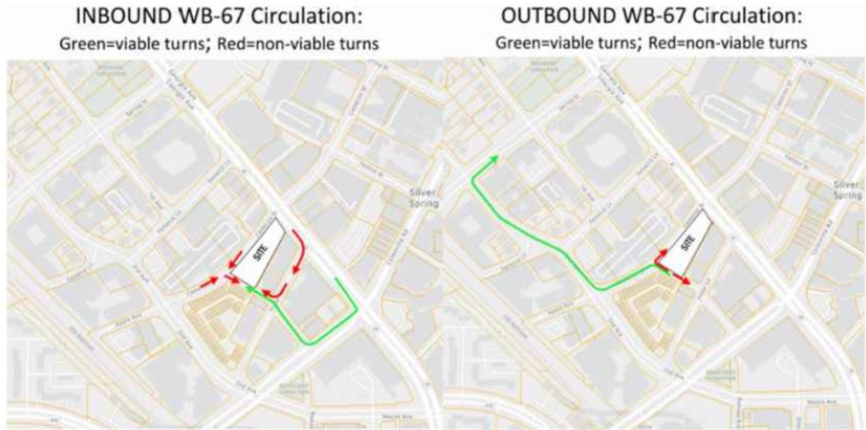
Figure 14: WB-67 Ingress and Egress Routes – Loading Management Plan
